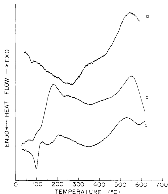
Figure 10. Differential scanning calorimetry (DSC) analyses of HPZ and borazine-modified HPZ: (a) HPZ; (b) 3; (c) 4.
